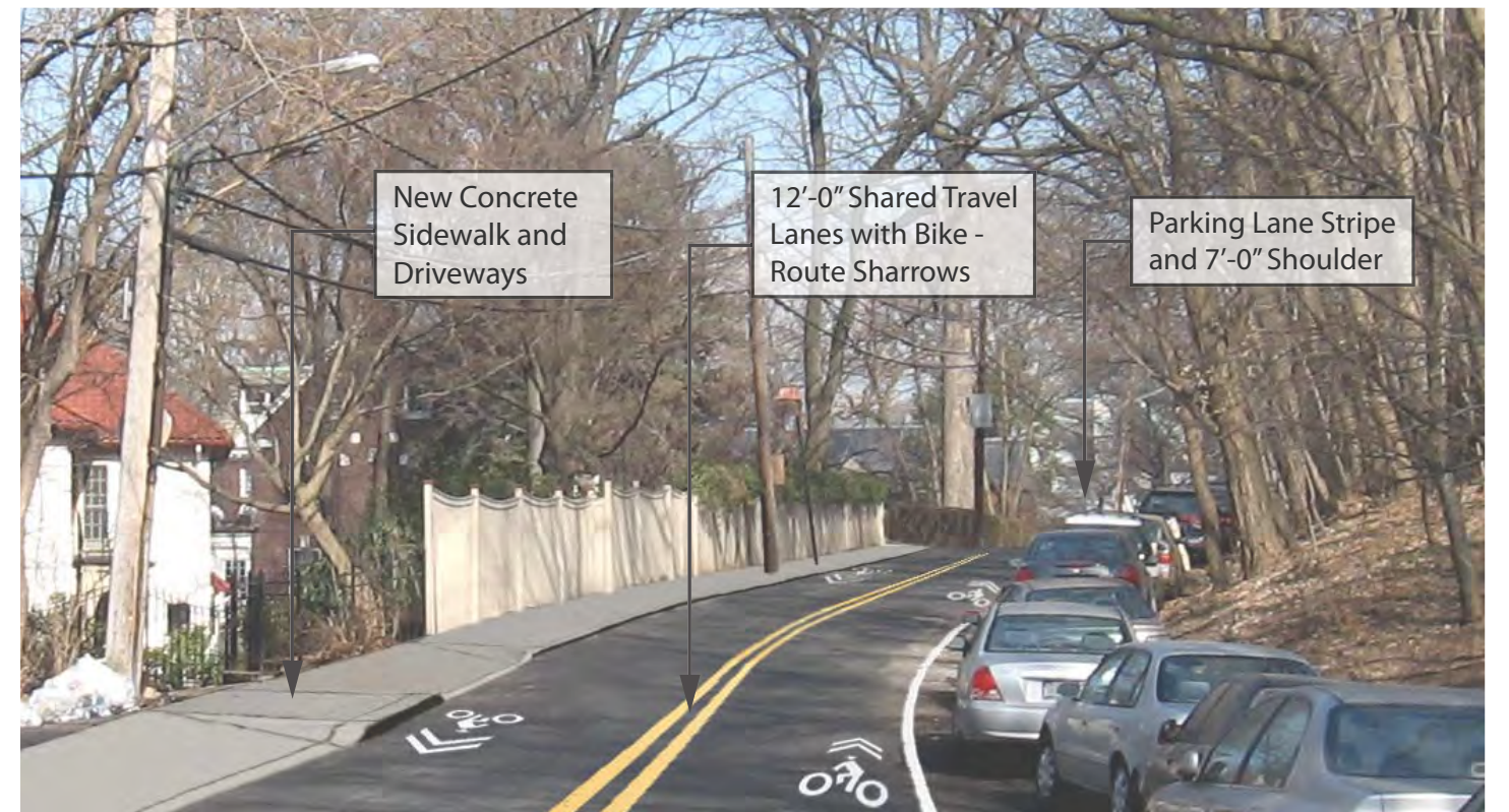
Proposed Conditions on Palisade Avenue
