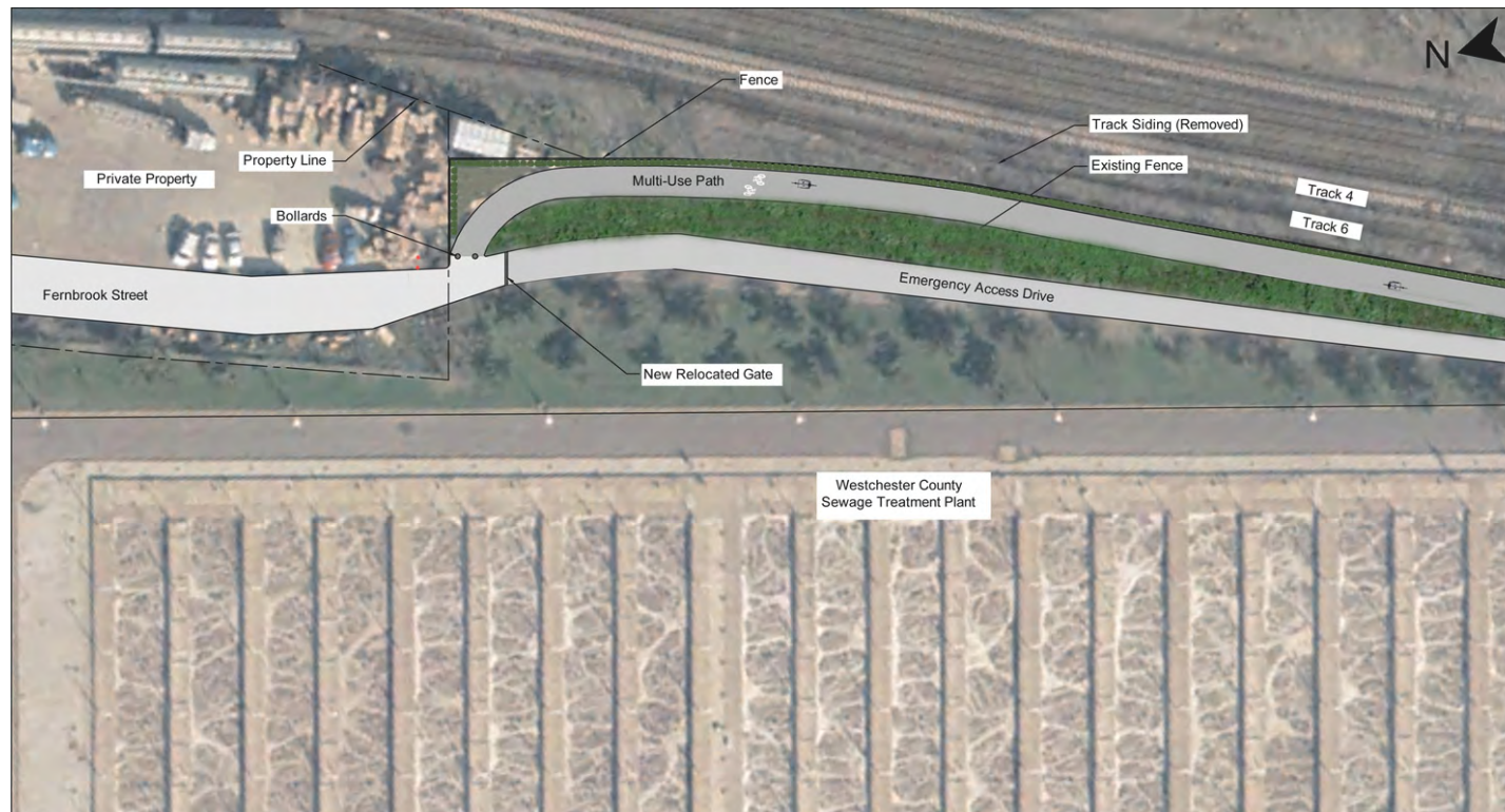
Conceptual Plan for Multi-Use Path Next to the Westchester Sewage Treatment Plant –Part 4 North. Proposed path exits MNR R.O.W. and cuts corner of Sewage Treatment Plant property to reach Fernbrook Street.
